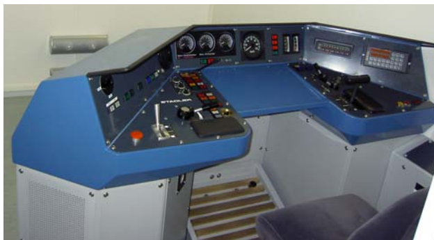
The same train protection system I/O devices with original equipment on the RAILplus simulator connected to PC via bus converters and RS232
