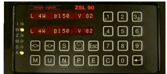
Input device of train protection ZSL90 of RBS and AAR reproduced on PC (control by mouse or touch-screen)
